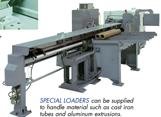
Stock diameter changeover is fast and easy with our electric screw-driven height adjustment.
