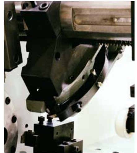
ID chamfer unit is used for deburring and chamfering.
