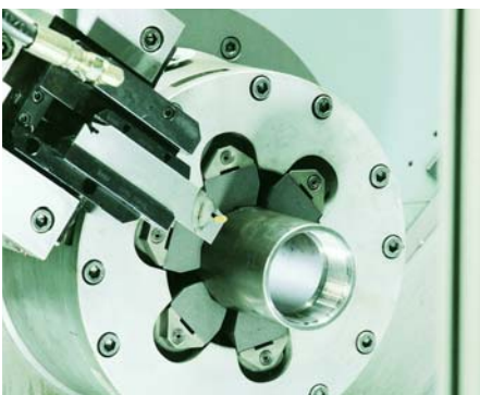
OVERHEAD CUT-OFF SLIDE Adds a third axis to allow for faster cycle times with overlap of slide use and saves a tool position on the turret or block type tooling.
