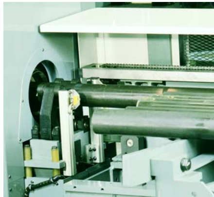
SELF CENTERING STEADY REST Self centering steady rest at rear of spindle supports work, keeps material centered.
